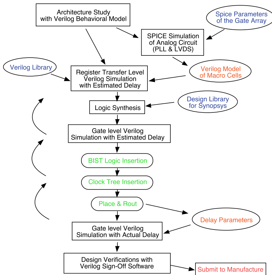
Fig. 42 Simplified design flow of the AMT chip.
