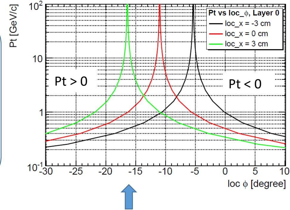
The sensor plane has +11.0 or 10.5 degrees with respect to the global coordinate. Due to geometrical constraints, any particles generated at IP have complex correlations among Pt values, Pt signs, local  $\phi$ , local x as well as stereo angles ( $\pm 40\text{mrad}$ ).
