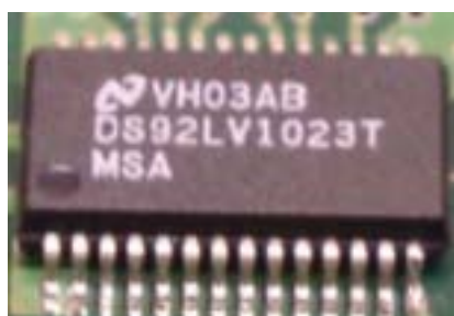
Figure 5-7 LVDS TX Chip (NS DS92LV1023)
