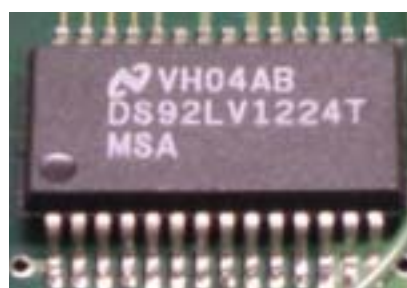
Figure 5-8 LVDS RX Chip (NS DS92LV1224)
