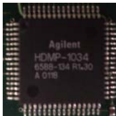
Figure 5-5 G-Link RX Chip (Agilent HDMP-1034)
