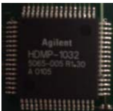
Figure 5-4 G-Link TX Chip (Agilent HDMP-1032)
