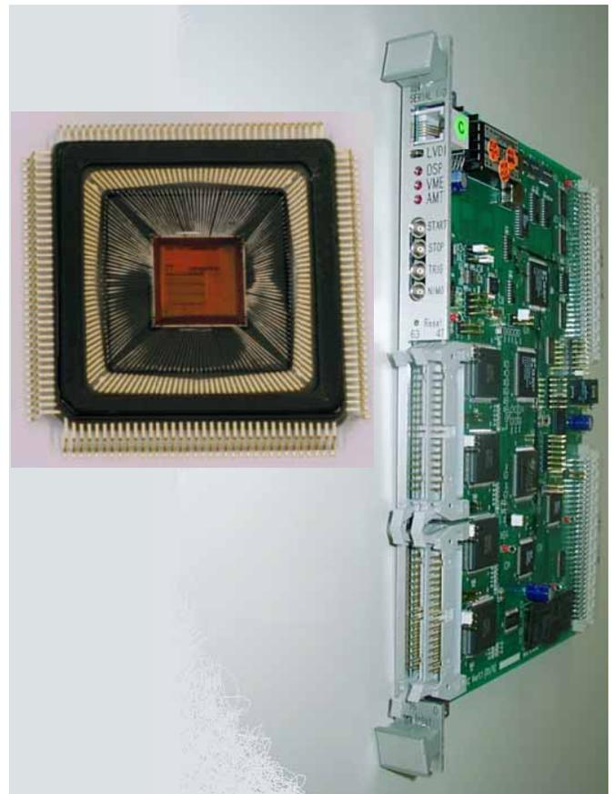
Fig. 1. Photograph of the AMT-2 chip and the AMT-VME module.
