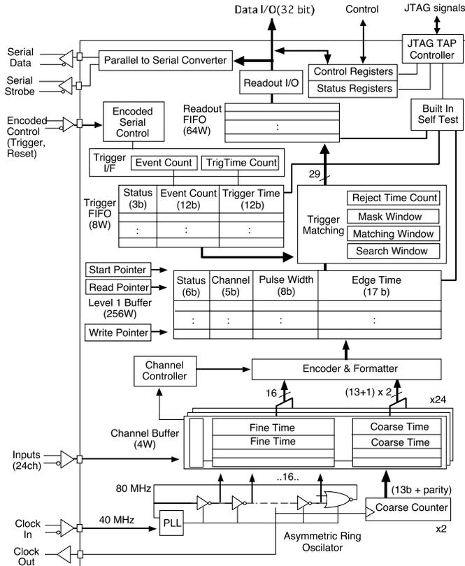
Fig. 3. Block diagram of the AMT-2 chip.
