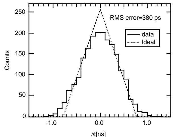
Fig. 7. Result of a time-resolution measurement (Time difference measurement between start and hit). Delay time between two pulses ranges from 0 ns to 1000ns in 0.1 ns step and fit by a line. The RMS error of the data is 380 ps. The dashed line shows ideal case distribution (digitization error only). The single-measurement error was derived to be about 270 ps.
