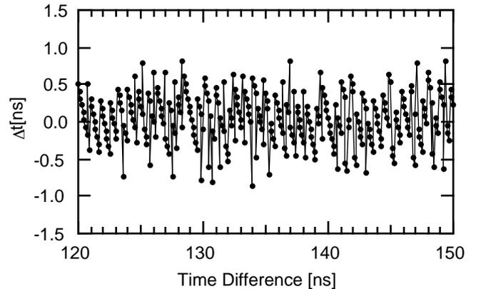
Fig. 6. Residual from a line fit. Data are taken in 0.1 ns step. A regular structure of digitization error (every 7~8 points) can be seen.
