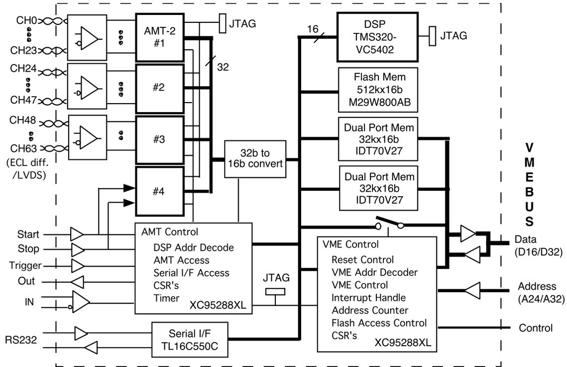
Fig. 2. Block diagram of the AMT-VME module.
