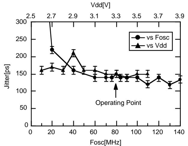
Fig. 5. PLL jitter vs. internal clock frequency and supply voltage. The operating point is shown by the arrow.
