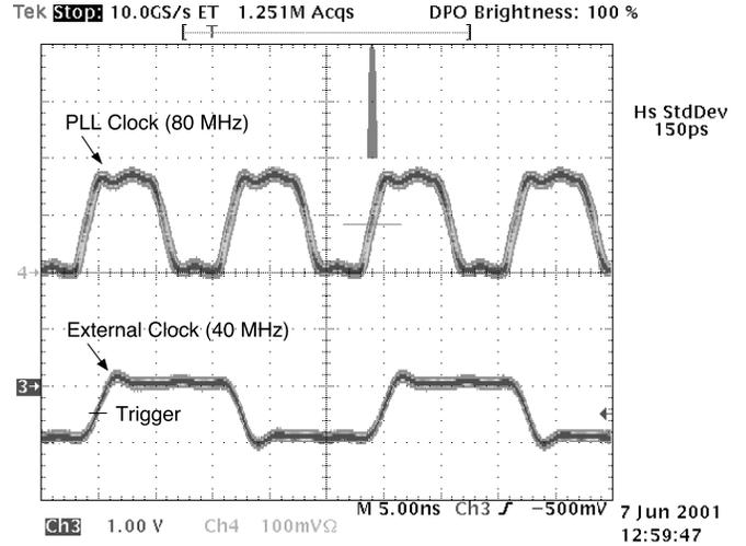
Fig. 4. PLL clock output waveform and jitter measurement. PLL clock jitter was measured relative to the external clock edge.
