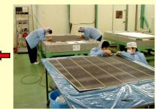
Inspection, cleaning, HV checking
