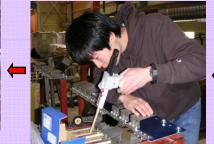
Fixing small leaks/final inspections
