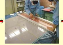
Applying epoxy for gluing
