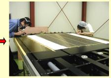
Soldering wires and washing
