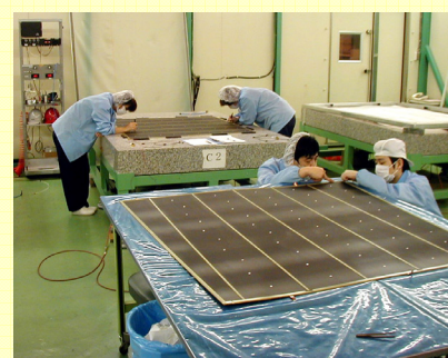
TGC construction at KEK
