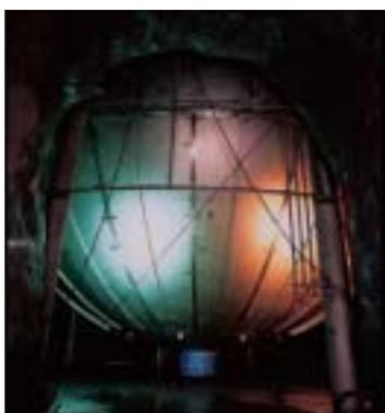
**KamLand** is the largest low-energy antineutrino detector with 1000 tons of liquid scintillator. It started operation in 2001 and already measured a flux decrease of antineutrinos from commercial nuclear reactors, supporting neutrino oscillation.
