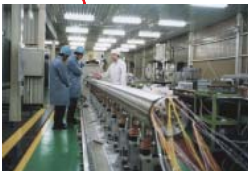
KEK developed and fabricated 18 superconducting quadrupole magnets which will focus the LHC beam at the ATLAS and CMS interaction points.
