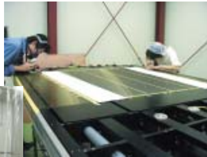
Soldering many thin wires. Japan built 1100 TGC chambers.
