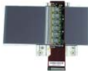
Four Si-sensors assembled with 1 micron accuracy. Japan made 980 SCT modules.
