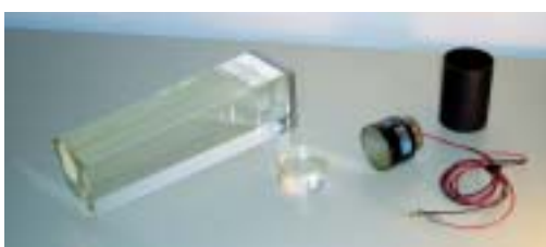
The components of the lead-glass counter.
