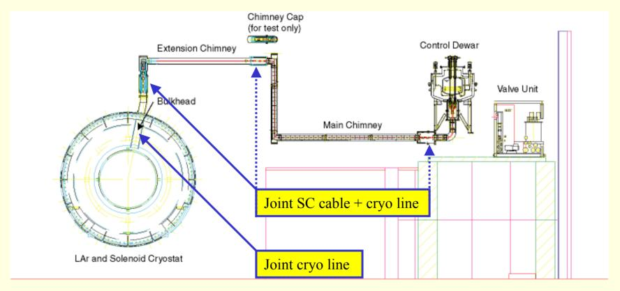
Conductor: 4 cables, main + side, supply & return Cryogenics: 4 tubes, 4.5K + 80K, supply & return
